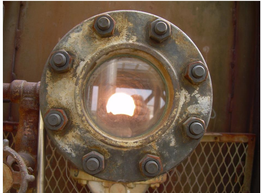
Material buildup in a sight port nozzle.
